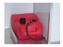
A large number of tools and equipment that you will be using require gasoline to work. Gasoline is a colorless liquid with a characteristic odor. It may be dyed yellow. Both gasoline liquid and vapors present a fire hazard. Gasoline liquid can accumulate a static charge by flow. The vapor is heavier than air and may spread long distances making distant ignition and flash back possible. Overexposure to gasoline vapors may
