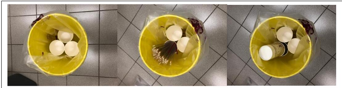
Figure 2. As you work in the BSC, have a cup/milk jar inside the BSC as a temporary waste container for the serological pipettes and tips. Once your work is completed, directly transfer the serological pipettes and tips into the designated yellow bin. Once the cups are full, cap the top with another cup and take down to SW111K as soon as possible.
