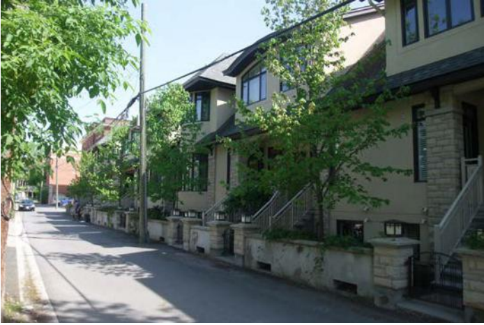
A narrow right-of-way serves as a traffic calming measure, allowing a residential laneway to function as a shared-street (Toronto, ON).
