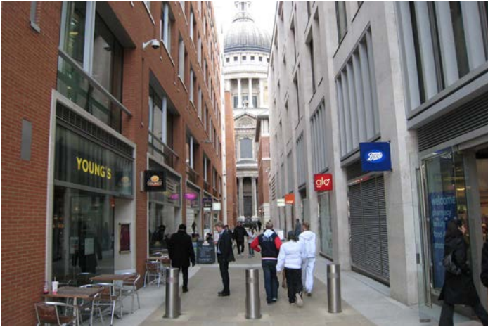
Traffic bollards maintain pedestrian priority along a commercial laneway while allowing vehicular access when required (Paternoster Square, London, UK).
