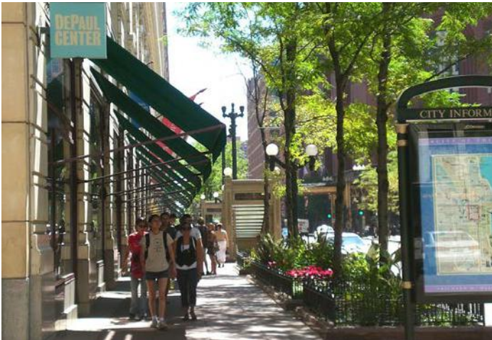
Retractable awnings provide flexible sun shelter which can be adjusted to desired level of sun exposure during different times of day and year (DePaul University, Chicago, IL).
