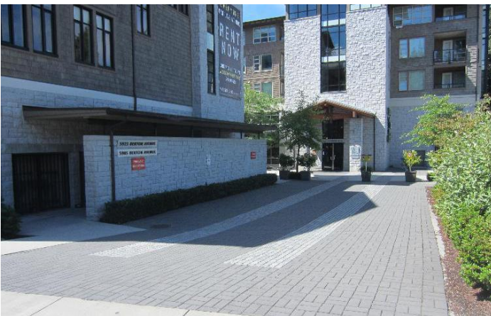
Screening and landscaping treatments can allow loading areas to function effectively in close proximity to building entrances and contribute to the open space network (UBC, Vancouver, BC).
