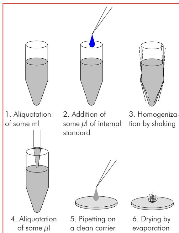
Figure 3: Preparation steps for the TXRF analysis of liquids
