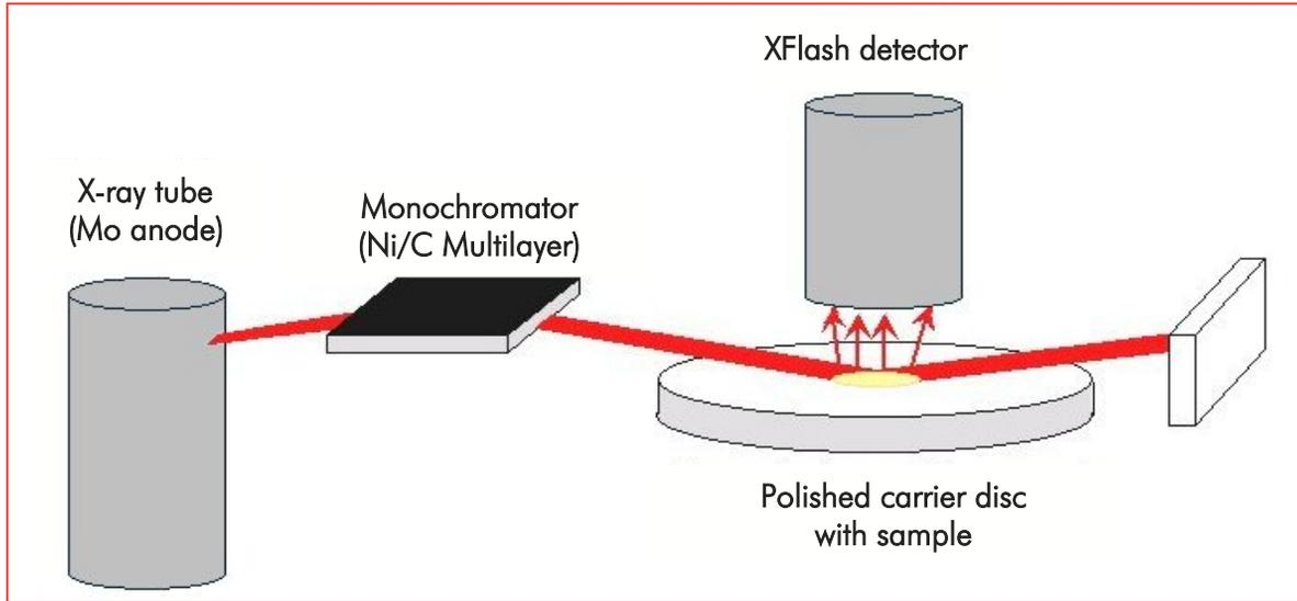
Figure 1: Schematic working principle of the S2 PICOFOX spectrometer
