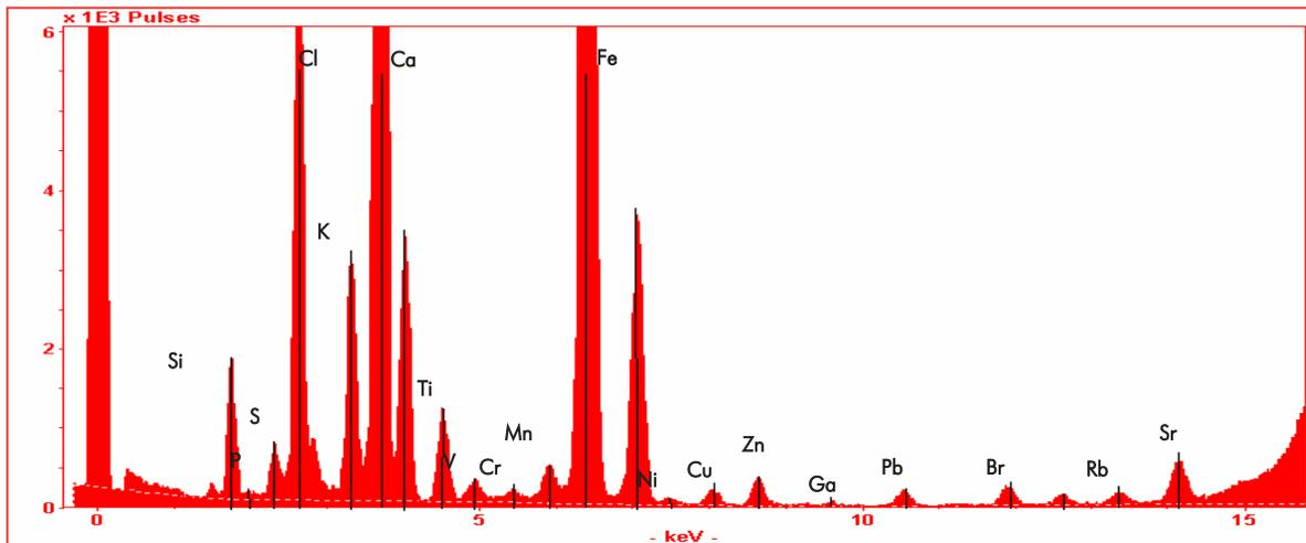
Figure 2. Typical energy dispersive spectra of the S2 PICOFOX
