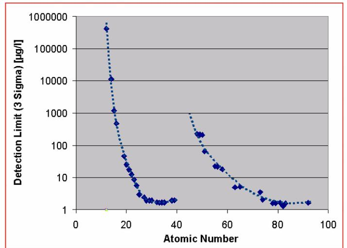
Figure 5: Low Limits of Detection for the S2 PICOFOX
