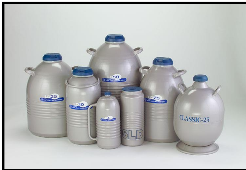
Figure 1. Examples of acceptable 'open top' flask or dewars for transferring of cryogenic liquids
