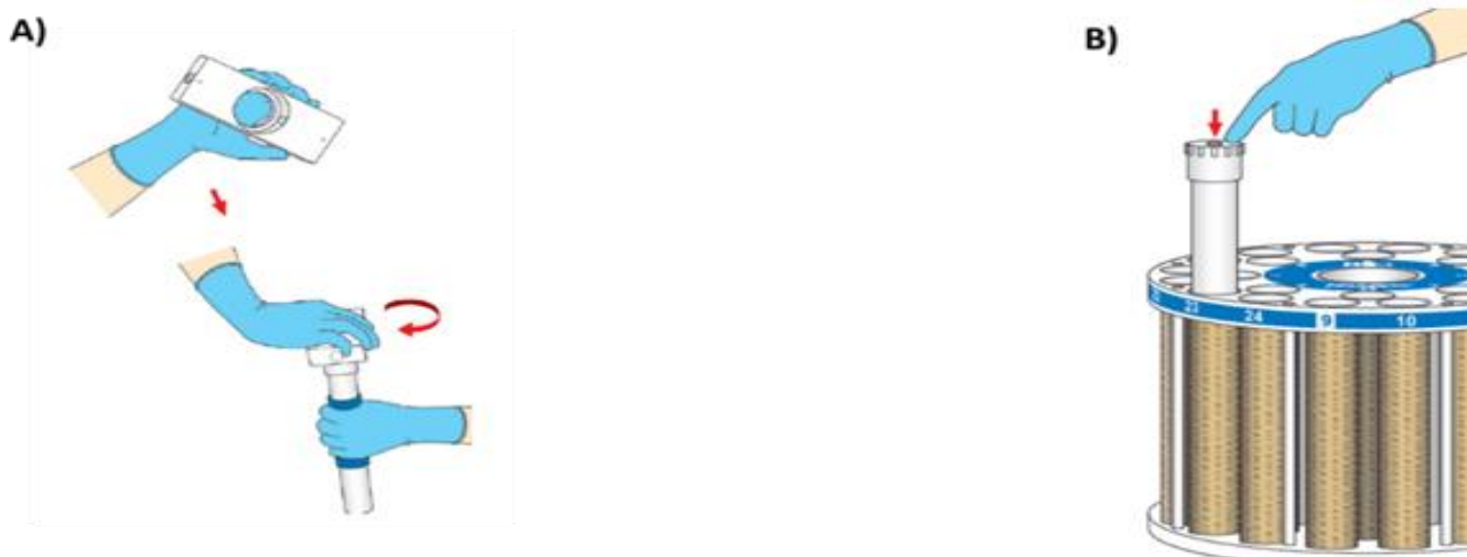
Figure 1. Schematic of A) how to properly use torque tool and B) proper insertion of sample vessels
