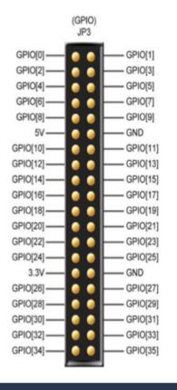
Instead of a constant 1 or o (5v or GND), connect to a GPIO port (General Purpose Input Output) Can turn the port on/off to control the circuit (output) Can read from the port to see if
