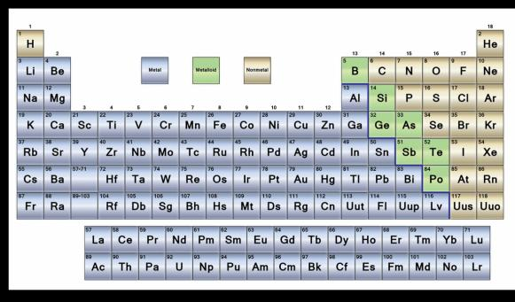
Semiconductor materials (silicon, germanium) straddle the boundary between conductors and insulators, behaving like one or the other, depending on factors like temperature and impurities in the material.
