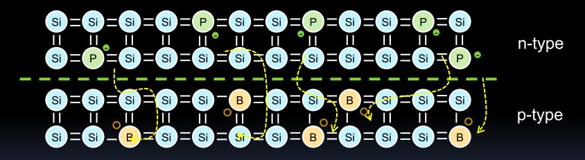
The electrons at the surface of the n-type material are drawn to the holes in the p-type.
