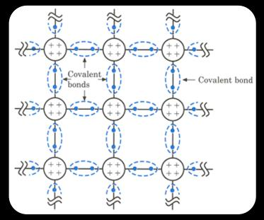
At room temperature, a weak current will flow through the material, much less than that of a conductor.
