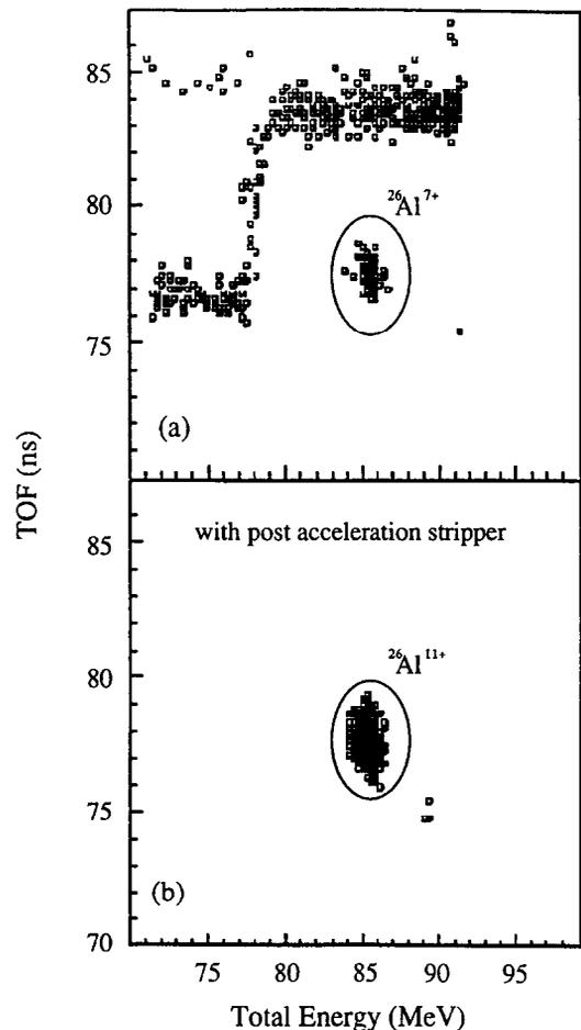
Fig. 1. Time of flight versus total energy for the ion detection system and an aluminum standard sample. (a) Spectrum without the post stripper measured with a beam attenuation of 40. (b) The beam attenuation was turned off for this measurement with the post stripper in place.
